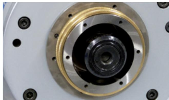
Taper hollow shaft with flat contact face
