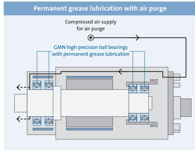
Permanent grease lubrication is characterized by low technical overhead and low life-cycle costs:
