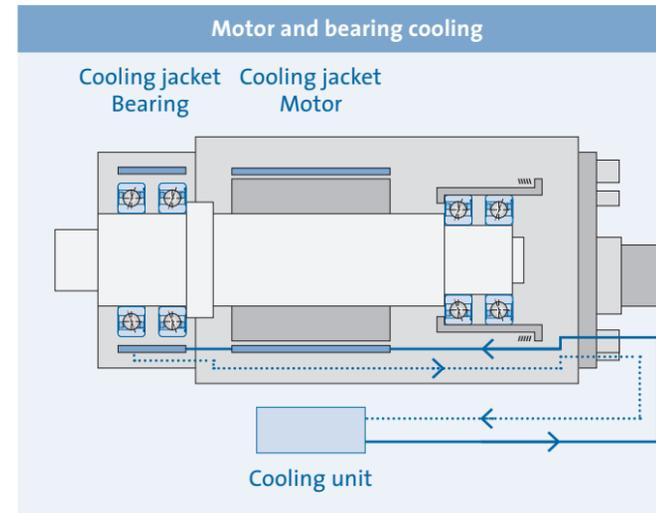
The reduction of operationally-induced heat development increases available spindle output performance, ensures maximum productivity and high processing quality.
