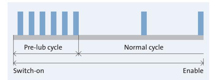
1. Start pre-lubrication (enable signal to operate the spindle not issued)
