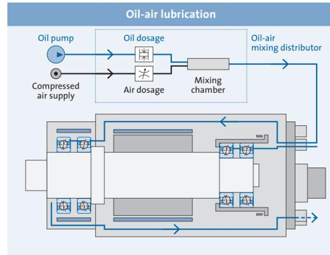
Oil-air lubrication guarantees utmost effectiveness with respect to consumption and lubricating effect at maximum speeds:
